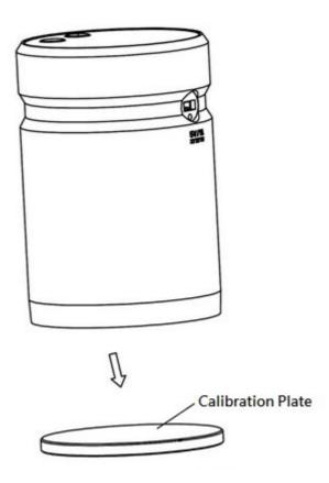
It is recommended to conduct calibration every 3 to 6 months. This product has a self-adaptability design. Frequent calibration does not help to increase accuracy.
